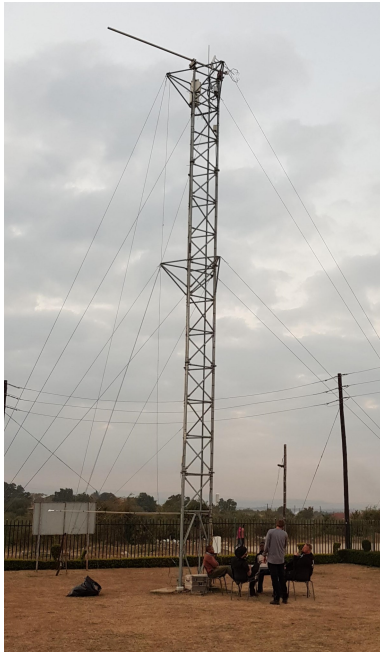
EMSAfrica Eddy Covariance tower at the Vuwani Science Resource Centre. Right: a practical solution for using a stone as counterweight to lift up replacement instruments. Photos Mari Bieri, Jens Jüdt.
