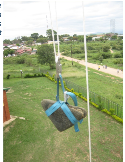
EMSAfrica Eddy Covariance tower at the Vuwani Science Resource Centre. Right: a practical solution for using a stone as counterweight to lift up replacement instruments. Photos Mari Bieri, Jens Jüdt.
