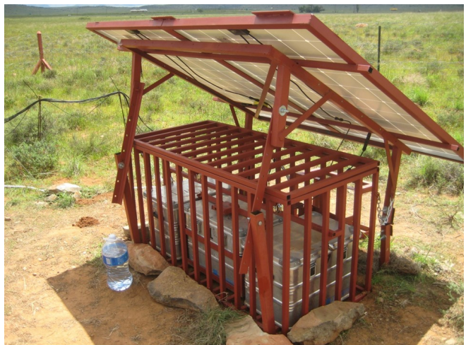
Middelburg EC tower during maintenance (left); new power setup with anti-theft steel cage and frame for solar panels (right) (Photos: Jens Jüdt).
